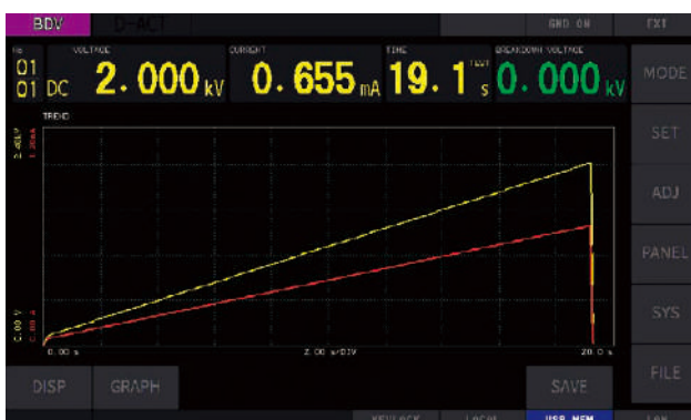
Example of continuous voltage rise test
