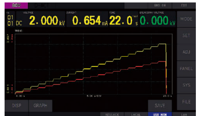
Example of stepped voltage rise testing
