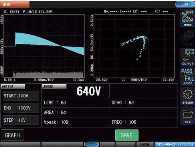
The above screenshot illustrates an example test conducted from 100 V to 1000 V using 10 V steps.
